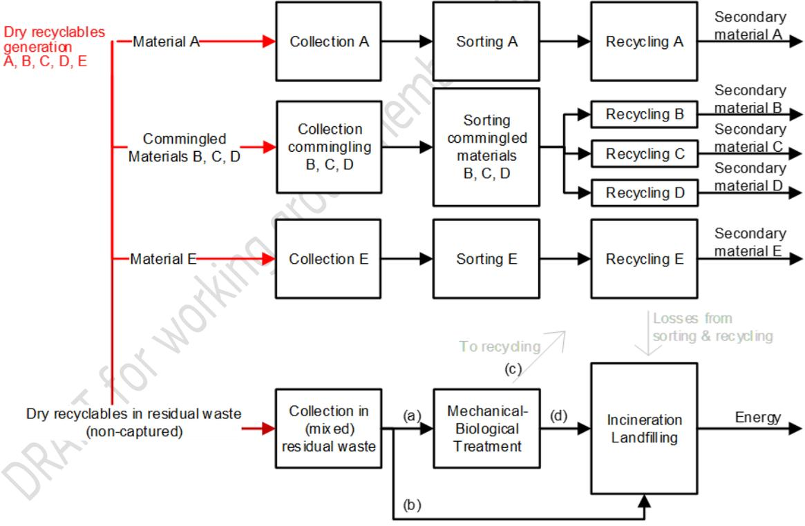
Figure 1. Exemplary illustration of a typical waste management scheme for management of dry recyclables. In this example, material A and E are collected separately, i.e. individually, while B, C,
